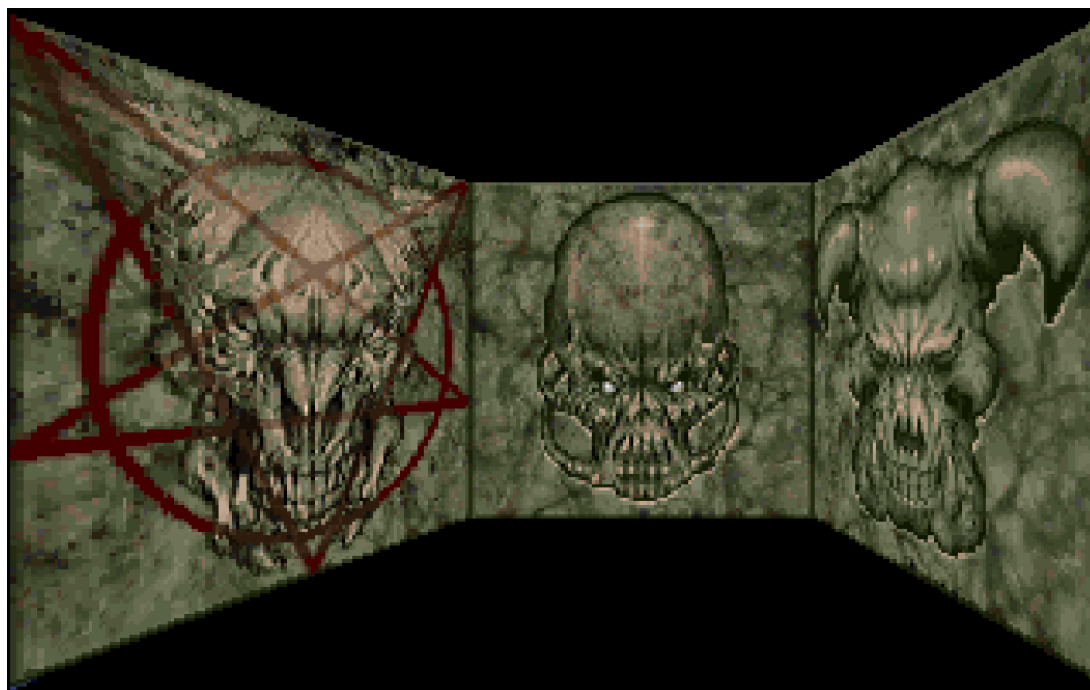
Above, distorted walls due to affine texturing. Below, perspective correct texturing.
