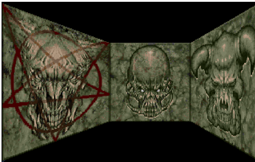
Above, distorted walls due to affine texturing. Below, perspective correct texturing.
