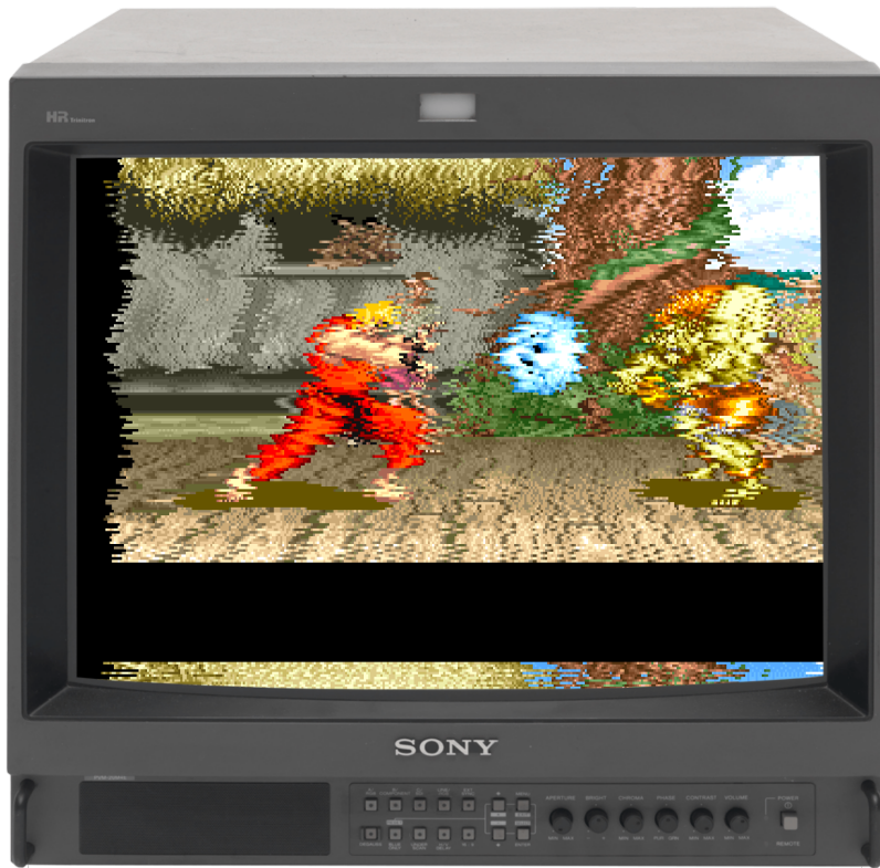
A desynced CRT. Lines are correct but not located where they should
