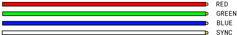
The four wires needed to drive a CRT
